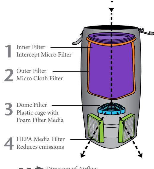
ProTeam's unique method of suction-vacuuming cleans carpets, hard floors, and other surfaces without stirring up dust – so the air stays cleaner, the furniture collects less dust, and operators can work without breathing unhealthy air.
