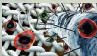
In this magnified view, the positively charged surface of MicroGard® attracts the negative charged bacteria. Due to the electrical attraction, the bacteria is drawn into the molecular spikes which puncture the bacteria membrane, eliminating it.
